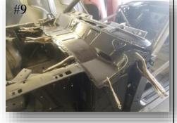
Outer cowl welded in place and plug welds ground down now ready to
