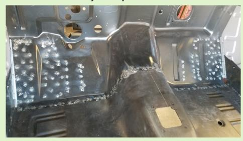
Firewall welded in place still needs a lot of grinding.
