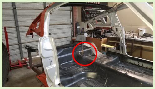
Brian marks the center of the floor and roof braces and uses a plumb bob to make sure it is lined up correctly before any welding.
