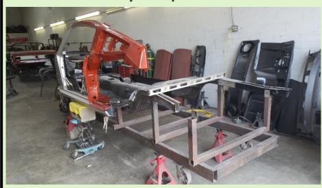
A long time ago we made a jig for a 1965 Mustang that attaches to the front and rear suspension points on a Mustang. This is how Brian can restore a Mustang that has a lot of new sheet metal and keep everything in the right place and level. The rear section of the frame rail will be replaced.
