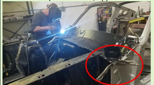
the front and rear roof braces, then clamped and screwed them together. Then he can begin to weld.
