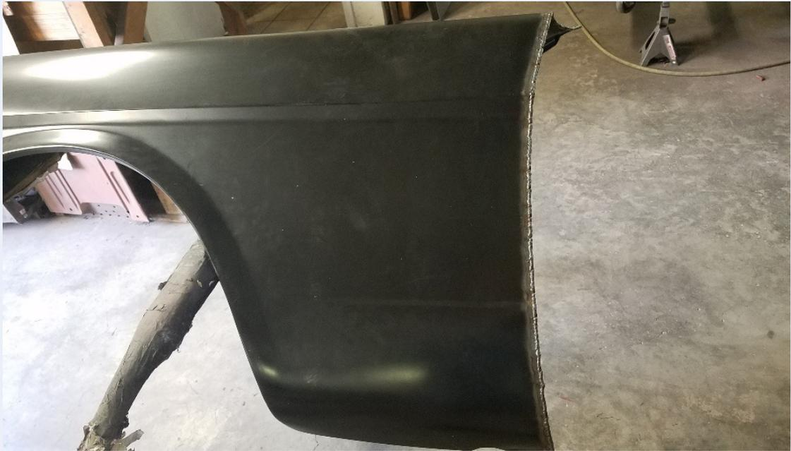
Brian test fit the doors and fenders and found out the gaps were off. To correct the problem he welds material on the fender or door and then grinds it down until he is satisfied with the gap.
