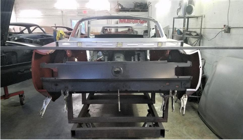
The taillight panel is test fit and Brian makes sure the top of the quarter panels are level.
