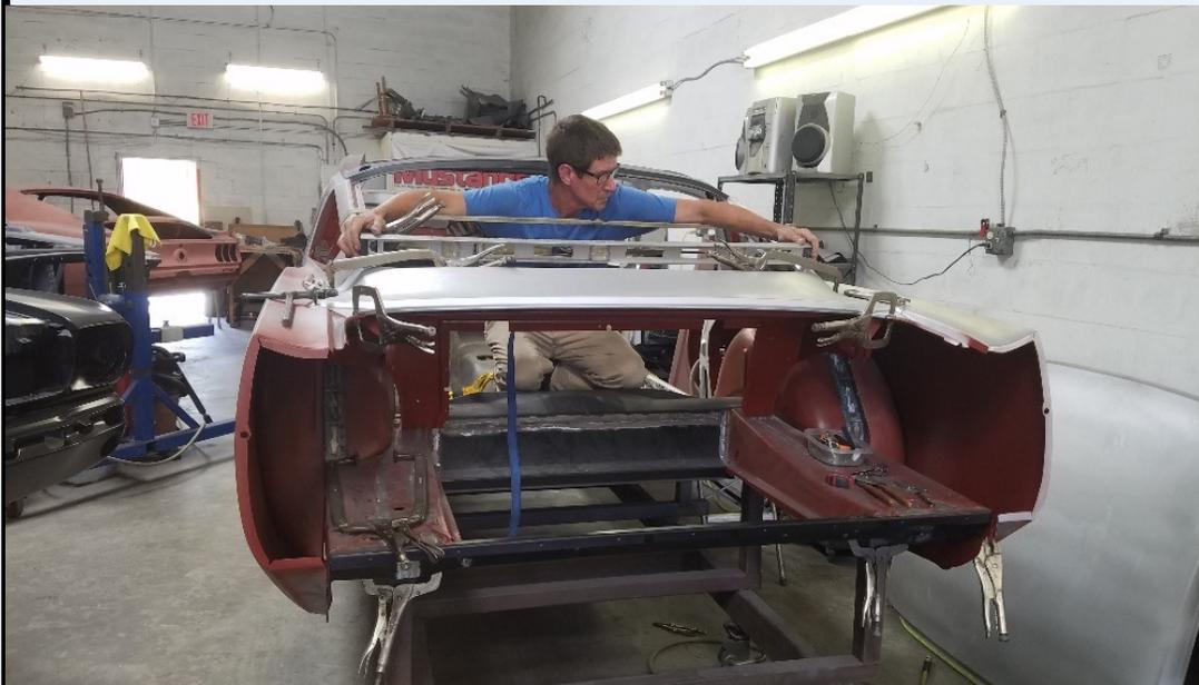
Brian does a lot of measuring and checking to make sure everything is level while it is screwed or clamped in place.
