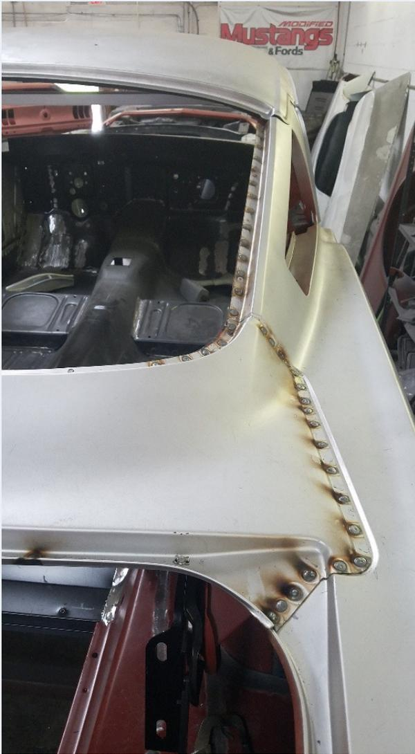
Quarter panel plug welded along with the deck lid filler panel.
