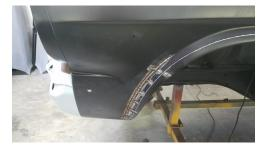
Left fender after it was welded back together.
