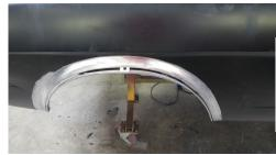
The front fender was cut but left attached at the bottom in the front and back and brought out 3/4" at the top and tack welded. I don't have a photo but he tack welded two more smaller braces. I wanted it to look like it was built by Ford but now you can use a larger and wider 17" or 18" wheel and tire.
