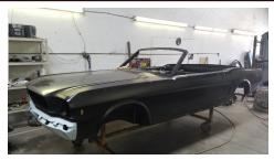
It is hard to get the fender and door gaps right on a 1965 Mustang because Ford never had a fender bracket behind the wheel opening until 1967. Brian made one for this project.
